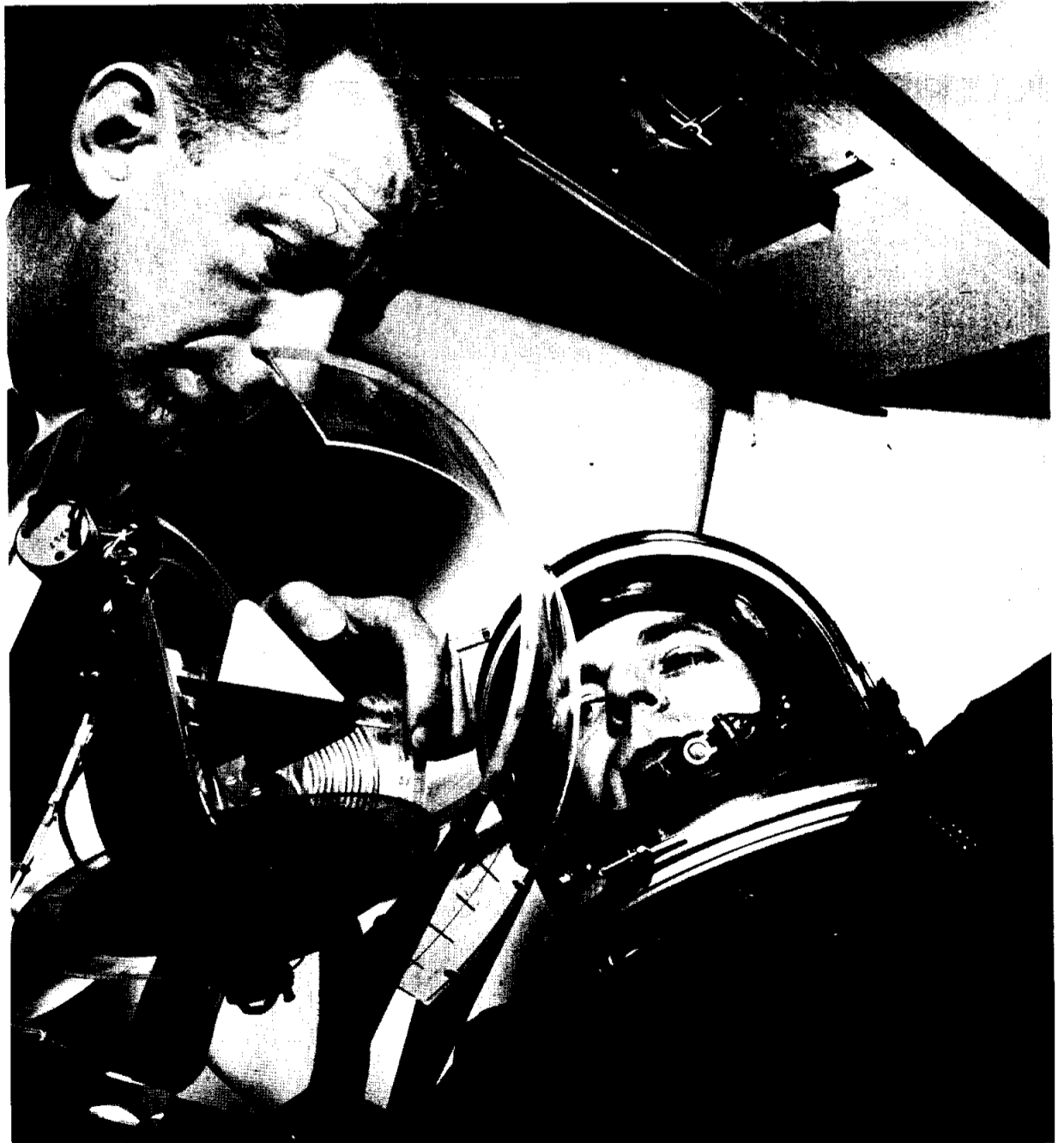
HOW DOES IT FEEL IN SPACE? — Down-to-earth engineers working on Project Apollo at Honeywell can now reach into "space" by simply thrusting an arm into a pressure suit glove affixed to a small plexiglass vacuum chamber. The simulation unit was built at the company's Aeronautical Division in Minneapolis for engineers who have never experienced the handicap of a pressurized spacesuit yet must design equipment for spacesuited astronauts.
