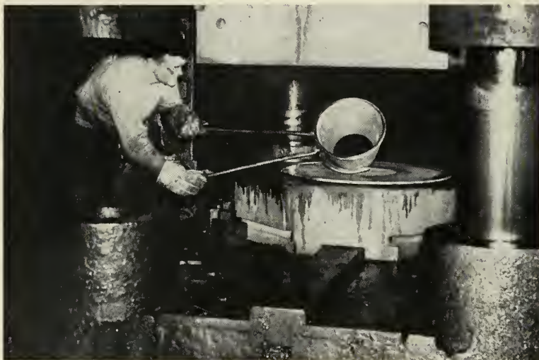
FIRST LARGE beryllium part ever forged successfully is on bed of 18,000-ton forging press at the Wyman-Gordon North Grafton, Mass., plant. Larger forging presses, including a 50,000-ton press, will be used to shape bigger and more complicated forms of beryllium in the future.
