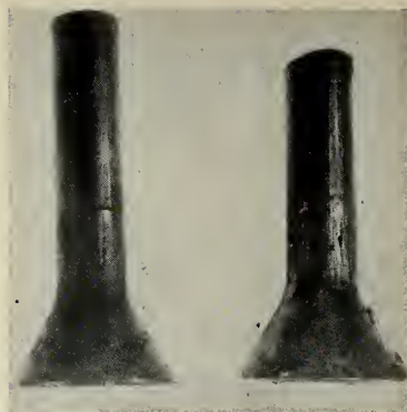
IMPACT extrusions of columbium-base alloys permit normal fabrication.
