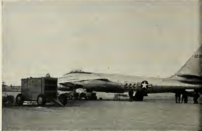
For a fast start, this Caterpillar Portable Electric Set is used to start jet engines and calibrate electronic systems at a SAC base.
