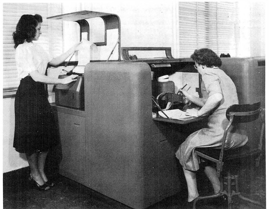
Shown above are two computers at the new Electric Calculator in the Langley Computing Section. The machine, built by the Bell Telephone Laboratories, fills an acute need for a fast, accurate solution to aerodynamic problems in high speed transonic research.
