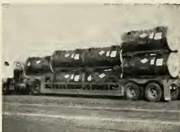
Note end sections reversed for empty shipment. Seven Harco containers with their integral ground handling trailers can be shipped in the same space required for three conventional containers.
