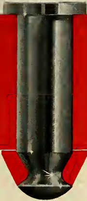
NOSE CONE SPLICE JOINTS ARE FASTENED WITH HS67 PINS, TYPE 431 STAINLESS STEEL, HEAT TREATED TO 125,000 PSI MINIMUM SHEAR. THE HS60M COLLARS ARE R MONEL.
