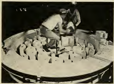
CERAMIC CORES —which had to hold their position under temperatures of about 2300°F—provided a ribbed, or honeycomb, design.
