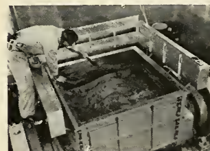
SOLIDS mixer by Baker Perkins is boosting propellant output for Thiokol Chemical Co. (p. 26)
