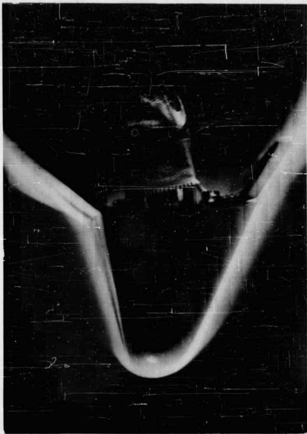
Model of entry vehicle in 12-inch shock tunnel, showing the luminous quality of the high-speed airstream.
