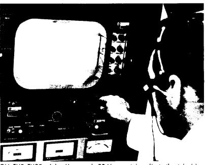
ON THE TUBE-John Hammond, BR-N, remotely adjusts the television camera viewing the RCS quad thrusters in the chamber.
