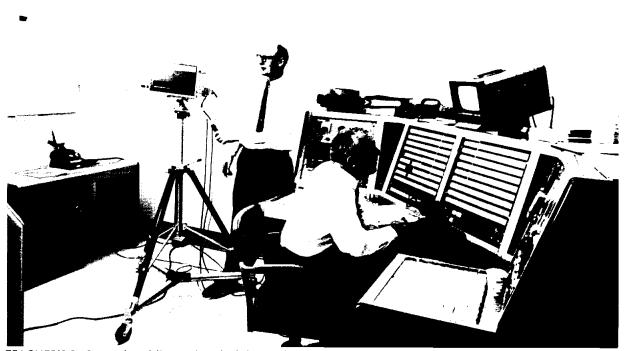
TEACHER'S DESK — Ed Middleton, head of the Cockpit Familiarization Group, mans the instructor's console from which switch positioning and other command module crew actions can be monitored. Sam Wenneker focuses the television camera on a schematic of the command module instrument panel which is fed to the rendezvous window monitors.
