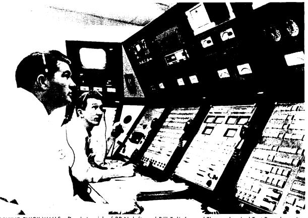
BEHIND THICK WALLS - Don Lotspeich of BR-N, left, and Bill Taliaferro of Thermochemical Test Branch monitor Apollo service module RCS thruster quad firings at the control panel in the Auxiliary Propulsion Test Facility. Closed-circuit television monitors show the thrusters in the 20-foot diameter subsystem test vacuum chamber. The control room is separated from the test chamber by foot-thick reinforced concrete walls.
