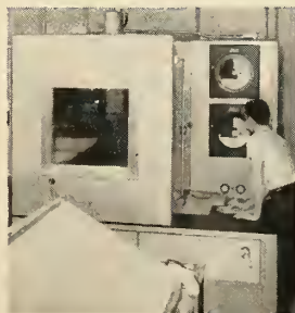
FH 36-5-5 TEMP.-ALT. — Temperature range —100°F. to +500°F., altitudes to 200,000 ft. (from atmospheric to 150,000 ft. in 11 minutes).
