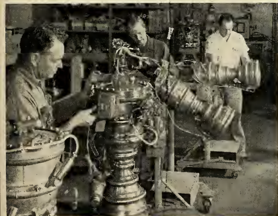
SHORT but powerful AR-2 liquid engines which were tested on FJ-4F are assembled at Rocketdyne.
