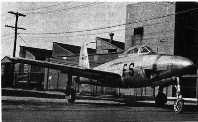
Working in cooperation with the NACA, Republic Aviation Corporation has developed flush side inlet ducts (shown on the left) on an experimental F-84, replacing the usual front ducts (shown on the right) normally
