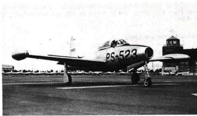
used on this plane. The development, intended to permit the installation of radar equipment in the nose section, was achieved with no performance loss to the airplane for interceptor missions.
