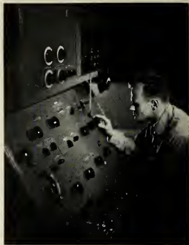
WENNER BRIDGE is used for calibrating these accurate, sealed double-wall 1-ohm standard resistors.
