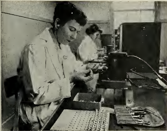
WELDING BRIDGE WIRES requires special tools, almost surgical cleanliness and care.
