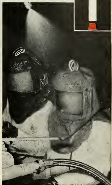
Nitric Acid Transfer to Missiles was made safe with the development of Aeroquip 610 KEL-F Hose Lines with stainless steel fittings. Picture above shows KEL-F Hose being used for fueling the Navy Vanguard.
