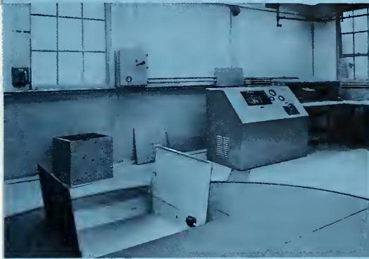
Giant centrifuge in special building at Ford Instrument can attain 60G's. Complete stable platforms—as well as components—are tested in this unit.
