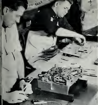
Missile-borne tape programmers being assembled. Continuous development in this field is under way at Ford.
