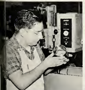
A special machine is used to mill irregular internal contours by an "electrical discharge" method, with extreme dimensional accuracy.
