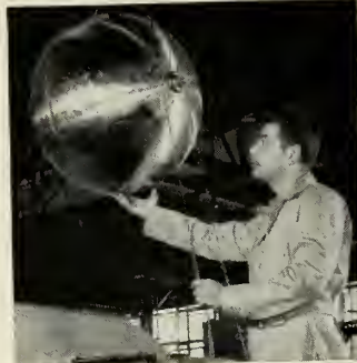
Successful titanium welding techniques have enabled fabricators to produce missile propellant storage bottles which resist internal pressures of 8000 psi at -300°F. This all-titanium bottle, produced by Rheem Manufacturing Company, Downey, Calif., is Ti-6Al-4V, fusion-welded in an argon atmosphere. Designers say use of titanium bottles can add up to 700 miles to the range of an IRBM.
