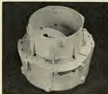
NEW K1X1 ALLOY sand casting is being used for new development missiles.
