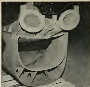
THE 150 LB. AIR-INTAKE of Regulus II is a magnesium alloy sand casting.
