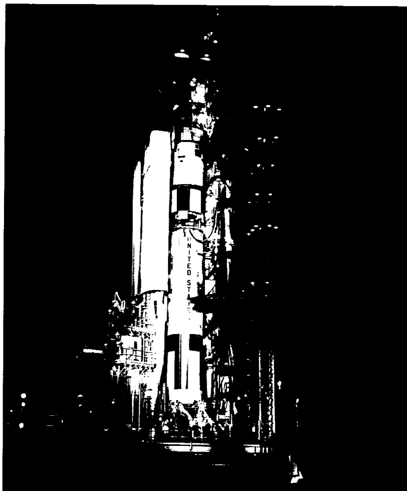
GEMINI LAUNCH VEHICLE - The first mating of the Gemini launch vehicle (a modified Air Force Titan II) took place early this month on Pad 19 at Cape Kennedy. The vehicle will be used later this year to launch the first unmanned Gemini spacecraft.
