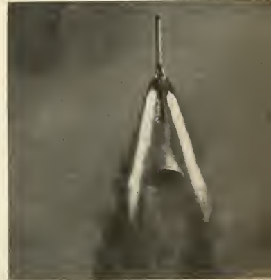
ESCAPE MECHANISM of the Project Mercury manned orbital capsule is tested at NASA's Pilotless Research Station at Wallops Island, Va. Mechanism is in the tripod arrangement on full-scale model weighing about one ton. Escape rockets lifted the capsule to 2250 feet where the tripod was ejected and a parachute lowered the capsule to the water where it was recovered by helicopter.
