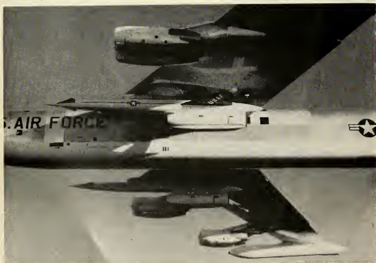
NORTH AMERICAN's Hound Dog air-to-ground missile carried by a Boeing B-52 jet of the Strategic Air Command. The new missile is currently in operational test.
