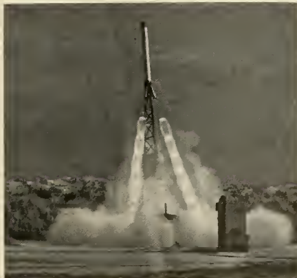
ESCAPE MECHANISM of the Project Mercury manned orbital capsule is tested at NASA's Pilotless Research Station at Wallops Island, Va. Mechanism is in the tripod arrangement on full-scale model weighing about one ton. Escape rockets lifted the capsule to 2250 feet where the tripod was ejected and a parachute lowered the capsule to the water where it was recovered by helicopter.
