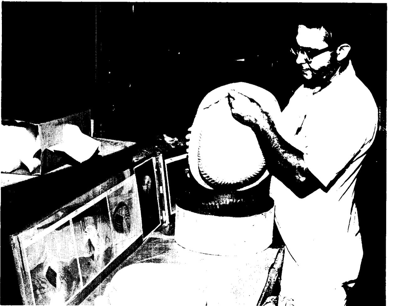
PARASAIL MODEL —John W. Heckler, experimental model maker in the plastics branch, disassembles the composite mould used in making a detailed scale model of the parasail. The model will have opening and closing louvers that are used to control descent and direction of the spacecraft by the astronaut.
