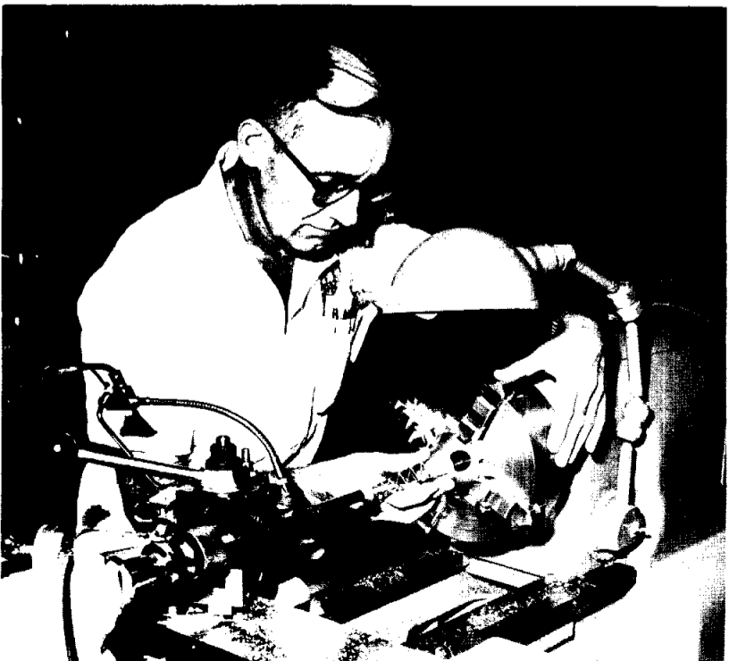
MODIFYING APOLLO MODEL —Jim O'Neill, metal model maker, modifies a model of the Apollo spacecraft to receive the escape tower. The model is to be used in wind tunnel tests. O'Neill also built the model of the centrifuge that is to be constructed at Clear Lake.
