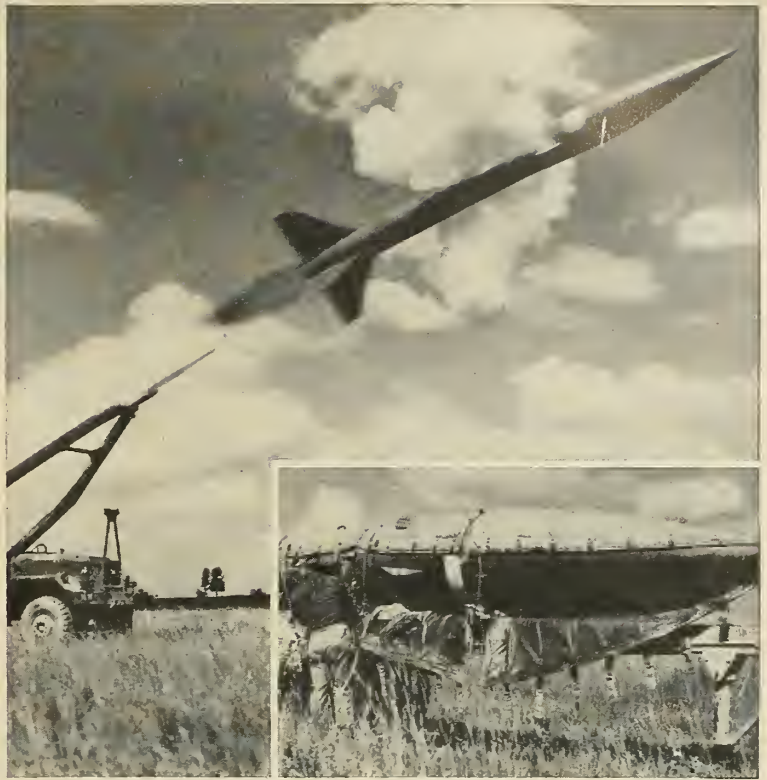
HONEST JOHN artillery rocket depends on G-E electric heating blanket (inset) to bring missile to uniform operating temperature before launching.
