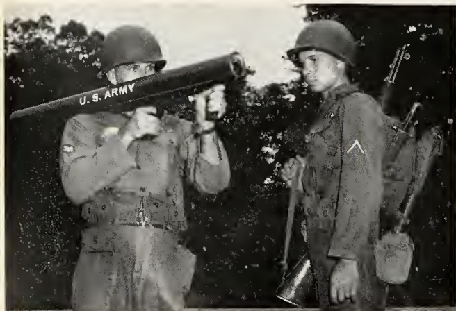
FOUR FOOT long Redeye has a diameter of about three inches and carries infra-red guidance.
