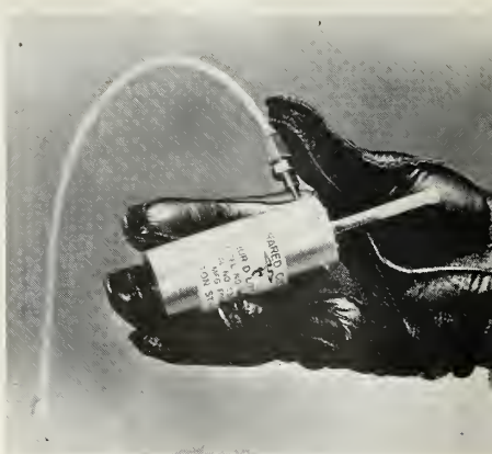
THIS Arthur D. Little-developed min-IR cooler is a low-pressure, closed-cycle refrigeration device developed for use with IR detection equipment.
