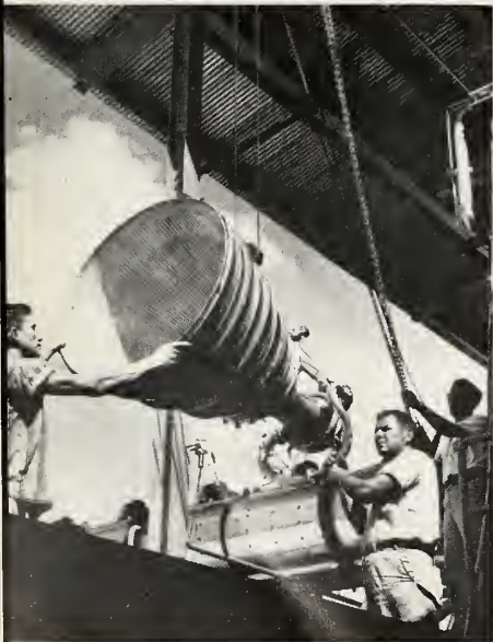
THRUST CHAMBER of XLR 115 is lifted onto test stand for static firing.
