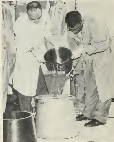
CASTING OF A truncated, cone-shaped portion of a re-entry vehicle thermal shield of new GE ablation material.
