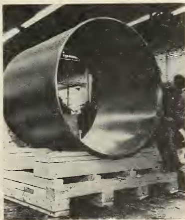
STEEL CASING fabricated for Aerojet by Kaiser Metal Products using hydro-spin process.
