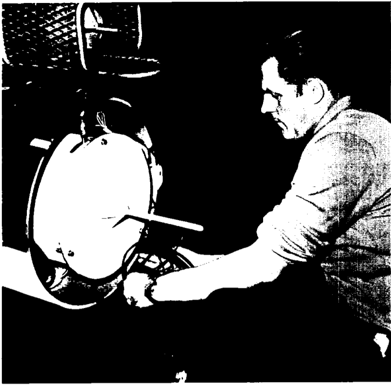
'PRE-FLIGHT' PREPARATION —Bob Koning installs instrumentation leads on Command/Service module portion of the one-third scale Apollo docking rig. Dynamics are measured in both mode of Apollo docking—transposition and docking of the Command Module with the Lunar Module/S-IVB after injection, and lunar orbit rendezvous and docking following the landing on the moon.
