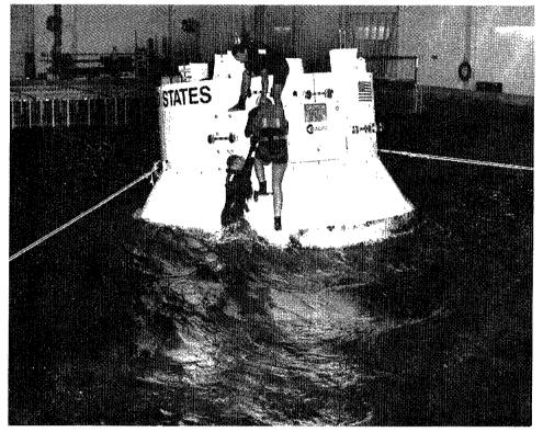
STAYING AFLOAT—Subjects test egress procedures during evaluation of the Buoyancy Assured Crew Return Vehicle test article in the wave tank at Texas A&M's Offshore Technology Research Center. Engineers studied how to remove an ill or deconditioned crewmember from the ACRV under various wave conditions.
