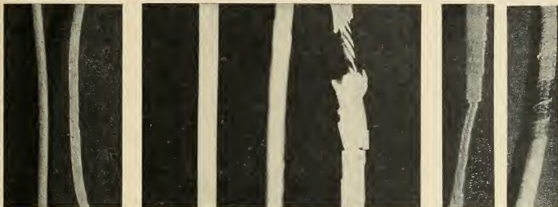
INSULATION resistance of Teflon coverings remained in the megohm range at high temperatures until thickness was sufficiently reduced by decomposition. Photo at left shows Sample 1a before and after test. Despite some thermal erosion, coating integrity was still maintained after ten minutes at 454°C. Insulation was maintained for more than 30 seconds (center); did not decompose until after 60 seconds (right). Photos at far right show construction of Sample 2 and results of 4½-minute exposure at 538°C. Slight thermal expansion is indicated by dark area.
