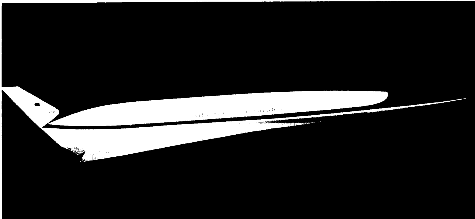
This is one example of how the Aerospace Plane might look once in operation. The hypersonic vehicle would be capable of speeds ranging from Mach 12 to Mach 25 and could make forays into low Earth orbit.
