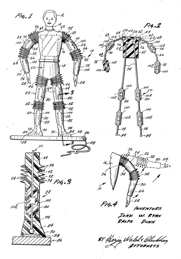
ADJUSTABLE FIGURE TOY HAVING IMPROVED ARMATURE MEANS
