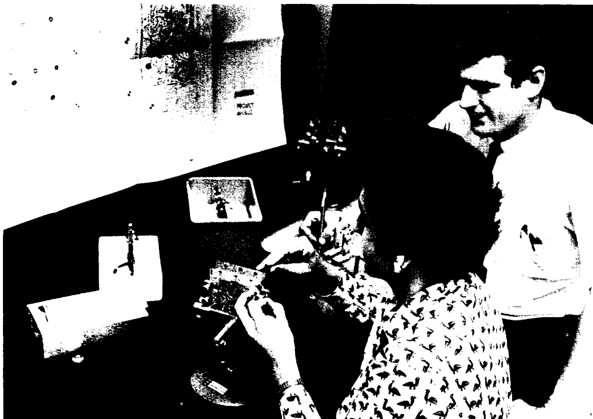
PHYSIOLOGICAL SIGNAL CONDITIONERS—Preassembly of physiological signal conditioners is performed by a Spacelabs technician with an in-process inspection.
