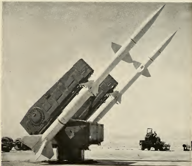
TWIN carriers in reloading position frame two supersonic surface-to-air Terriers .
