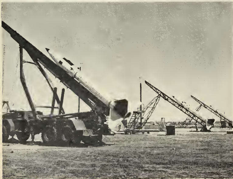
SIX-MAN crew can handle and fire Honest John , shown on its self-propelled launcher.
