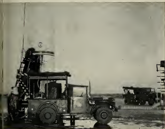
HYDROGEN peroxide service truck is part of support equipment for Redstone .
