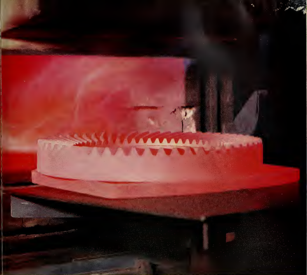
Large concave spiral bevel gear is so distortion free after heat treatment that it meets the highest aircraft gearing standards without subsequent tooth grinding.
