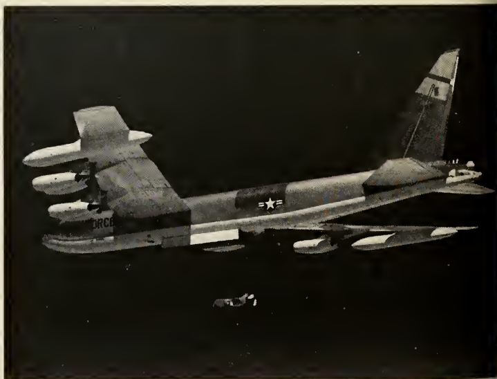
B-52 launches a GAM-72 Quail , designed to confuse the defenses of an enemy
