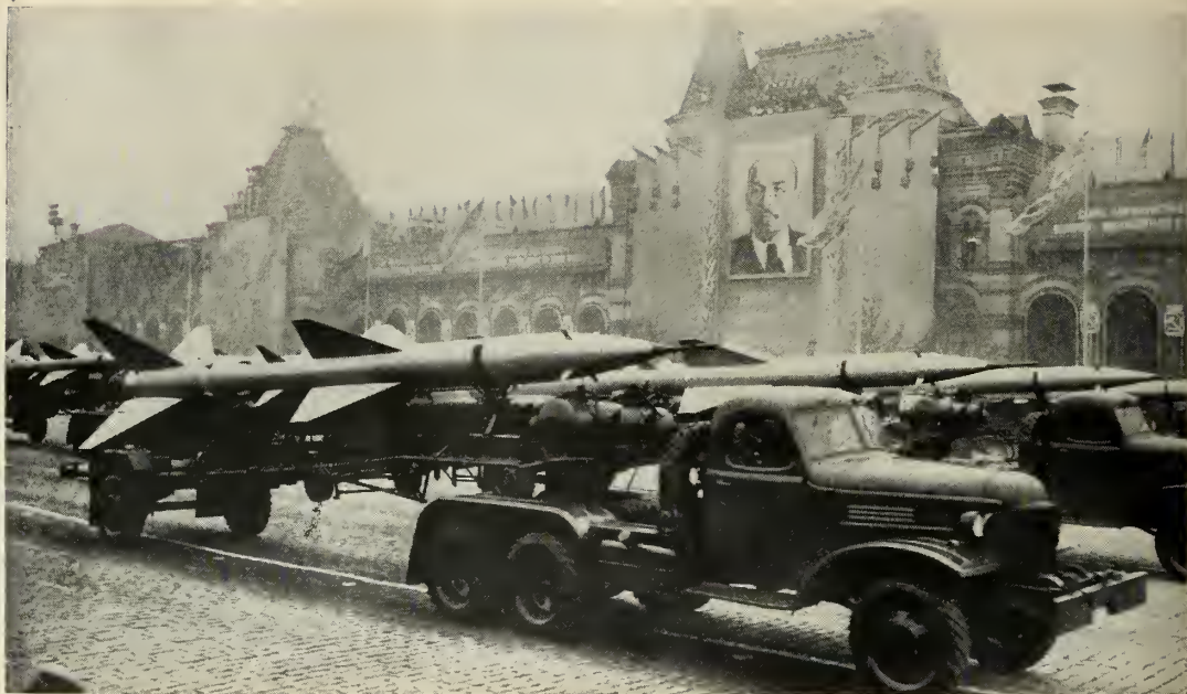
TWO-STAGE surface-to-air M-2 travels at better than 1500 mph and is guided by both radar and infrared.
