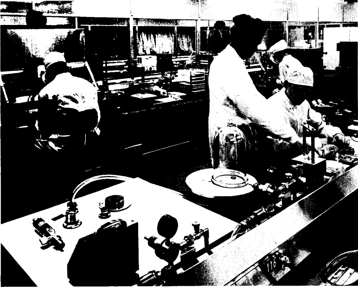
Gyro instruments for the Apollo navigation and guidance system will be assembled here. This is just one of AC's super-clean areas necessary for the building of inertial navigation and guidance systems.
