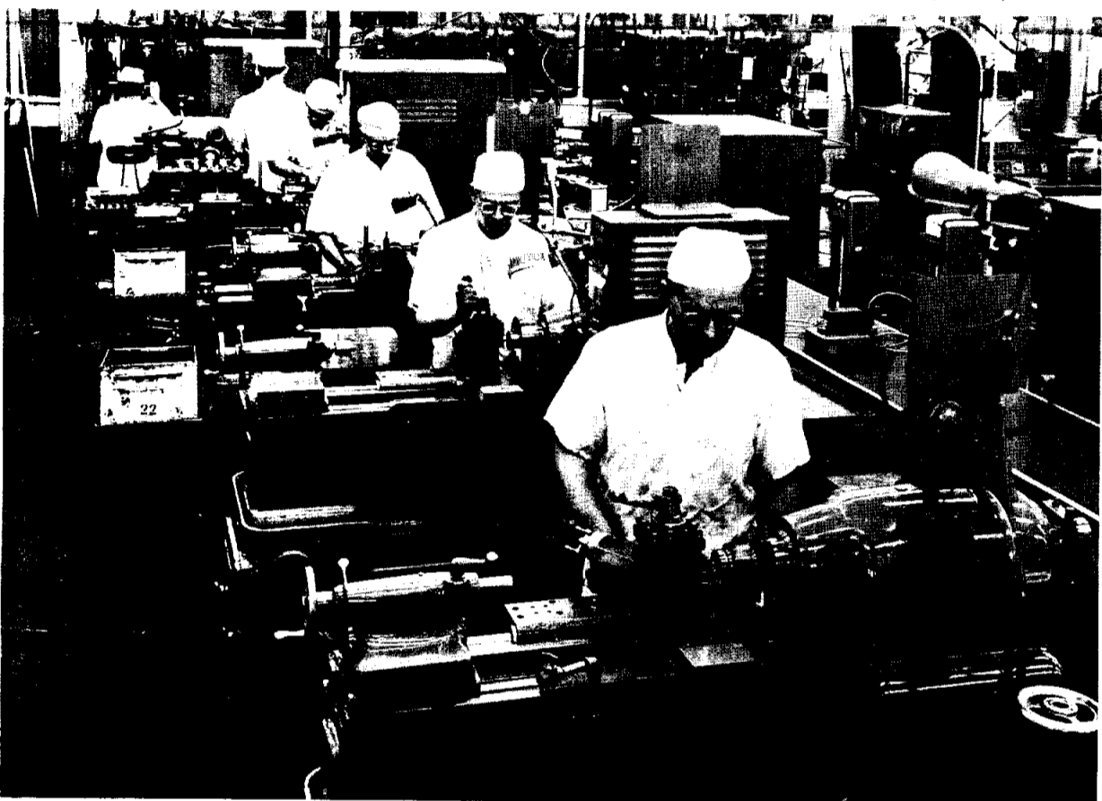
In this modern beryllium machining area, inertial components for the Apollo guidance and navigation system will be manufactured. This is a temperature-controlled area where the air is continually changed and tested.
