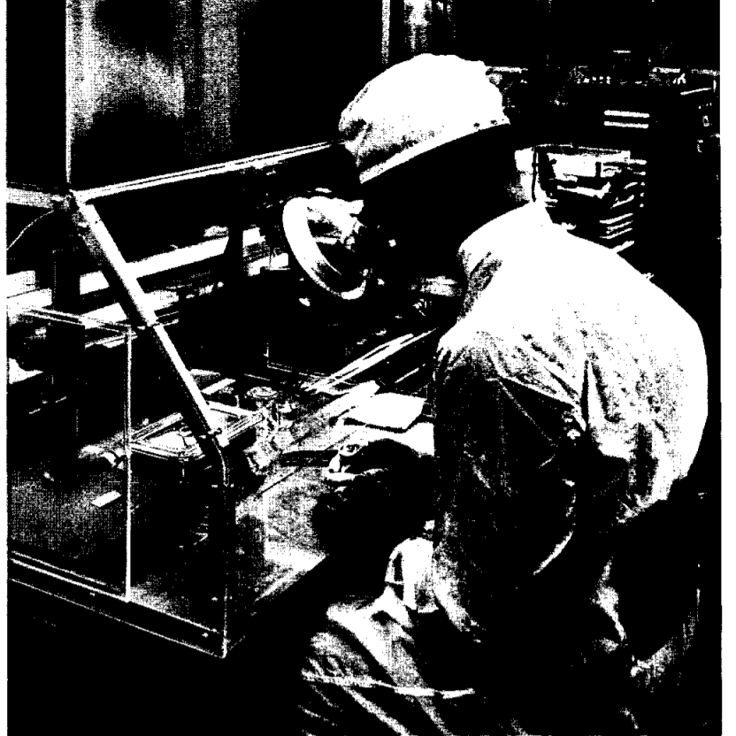
A TECHNICIAN in one of AC-Milwaukee's super-clean assembly rooms examines the wheel assembly of an Apollo gyro. Meticulous care to see that each part of the Apollo gyro is free from burrs or other contaminants, is taken.
