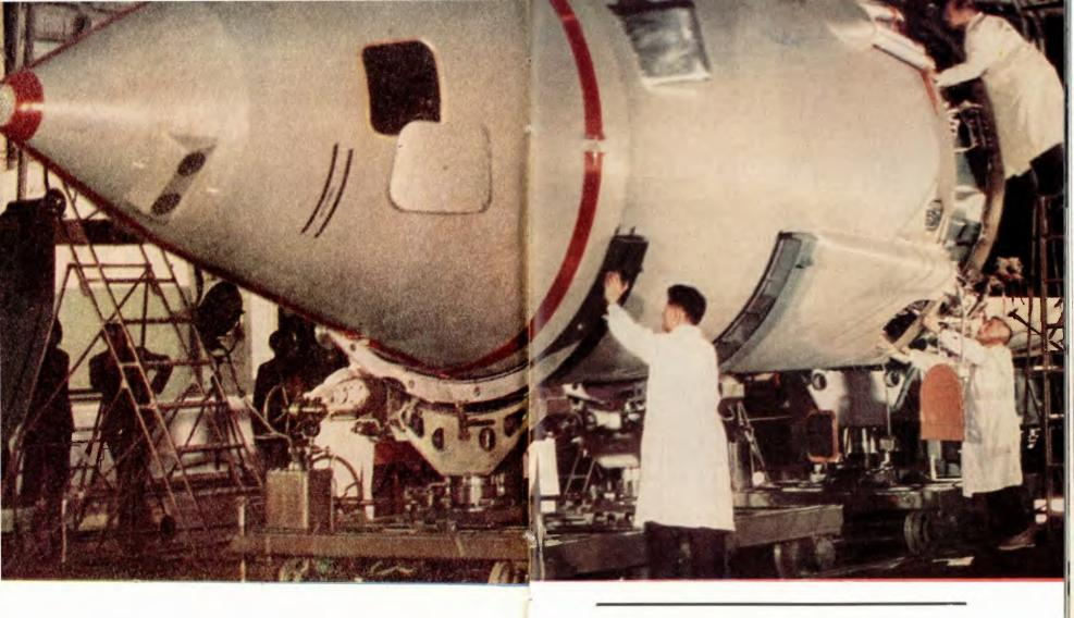
The ballistic cap being fitted to the spaceship in the assembly shop. Closer to the cone of the ballistic cap is the descent control apparatus which houses the cosmonaut's capsule and an instrument compartment behind it. During the boosting stage of the flight the ballistic cap protects the ship as she passes through the dense layers of the atmosphere. Then the cap is jettisoned.
