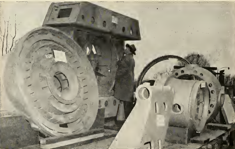
BULKY PARTS of Nike-Ajax tracking assembly look heavy, but weigh 3,200 lbs.
