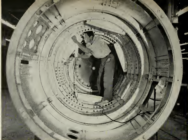
FORWARD SECTION of Redstone missile, shown here, would have been used in Army's Project Adam proposal to rocket a man 150 miles into space. "Man-in-space" portion has been cancelled because of conflict with X-15 program.
