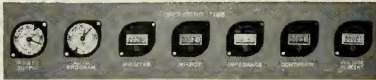
The illustration shows how the operating time of various sections of an electronic console can be monitored.
