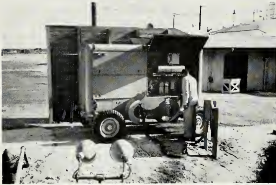
Snork Missile is powered by this Caterpillar Electric Set, photographed at Cape Canaveral, Florida. Full designation: Caterpillar 60 KW 400-cycle 120-208 Voltage Low Silhouette Portable Ground Support Unit with Precision Control Regulation.
