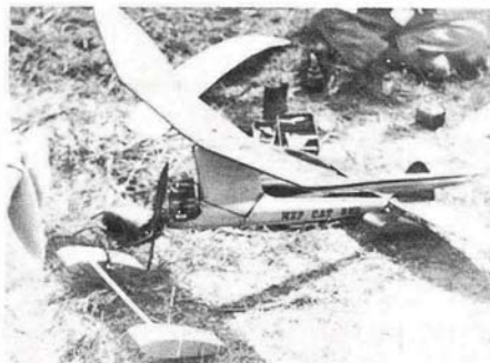
Shown above is the "Hep-Cat #2" fitted with floats to be used as a Hydro job.
