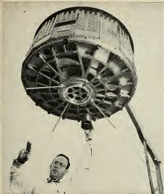
COMPLETE SATELLITE is positioned for tests of solar cell power supply at RCA Astro-Electric Products Div., Princeton, N.J., where Tiros and its ground system were built for NASA under Army direction, by Asst. Project Mgr. A. Schnapf.
