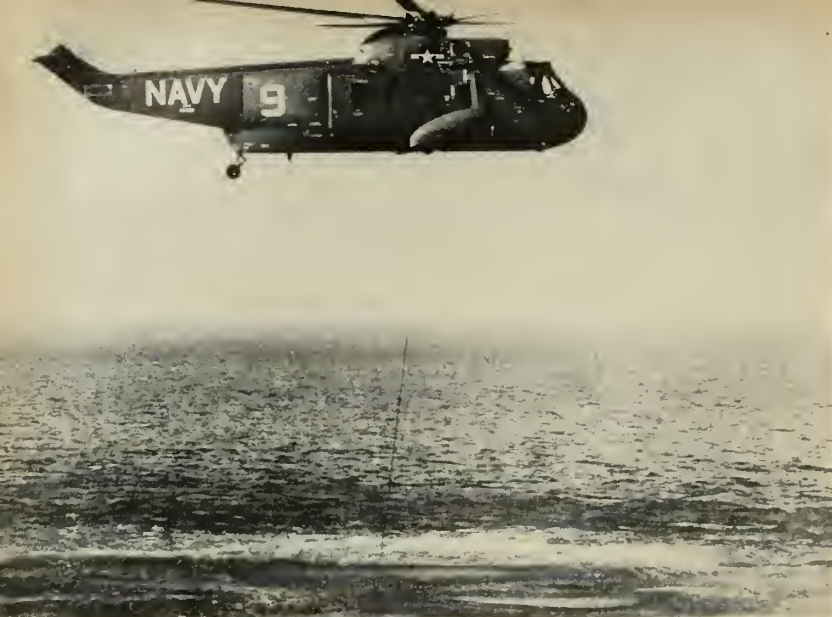
WORLD'S LARGEST amphibious helicopter, Sikorsky's HSS-2, conducts dip tests of its sonar detection gear.
