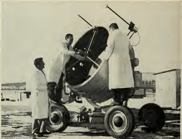
ARMY SURPLUS searchlight was converted by engineers at Thiokol Chemical's Reaction Motors Division to a solar furnace for testing material properties at high temperature. Dr. Stanley Tannenbaum, Dr. Frank Loprest and Steven Tunkel are shown adjusting the furnace, which can produce temperatures of 6300°F at ¼-in. focal spot. Electronic couplings enable furnace to track sun automatically and control temperature at sample.
